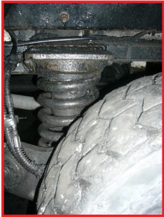
Hardy Spicer Rubber Springs are used to assist the coil spring carry more weight evenly.
