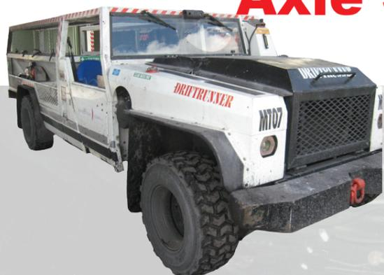
Manufactured in Europe using high quality steel to withstand the rigorous conditions of the underground coal mining for the Australian market.
