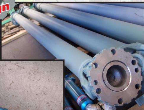
Joy Shuttle Car Shafts Upgraded UJ Design from the CV design
