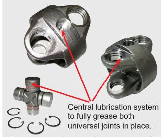
The system works through grease tracks in the yokes and holes in the universal joint caps which is greased through 2 grease nipples opposite each other.
